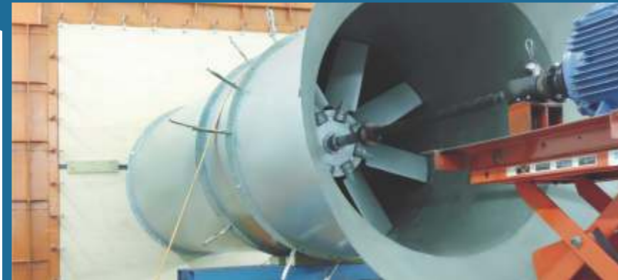
Testing of 'Ventech' Fan at AMCA accredited laboratory in Malaysia
